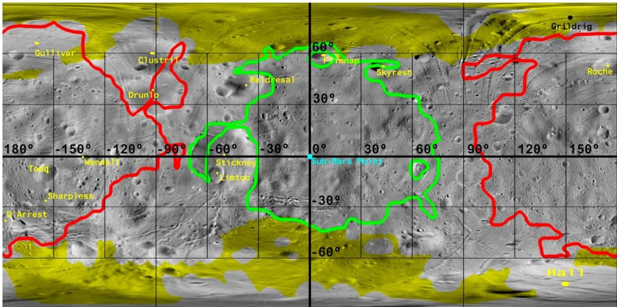
**Figure 8. Map of Phobos showing regions of continuous sunlight in yellow. The region inside the green boundary has line of sight to the full disk of Mars, while the region between green and red boundaries has visibility to parts of Mars. Underlying photomosaic courtesy Phil Stooke.**
