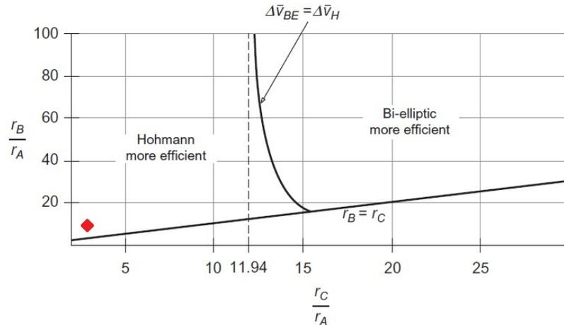
Figure 17: Orbits for which the bi-elliptic transfer is either less efficient or more efficient than the Hohmann transfer ( $r_A$  referring to the starting orbit,  $r_b$  referring to the bi-elliptic apoapsis,  $r_c$  referring to the final orbit; Curtis, 2010).
