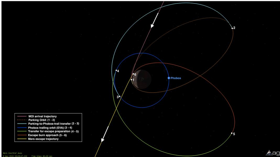
Figure 11: A comprehensive photo of space mission orbital maneuvers performed in an Areocentric orbit. The two white arrows indicate incoming and outgoing asymptotes.
