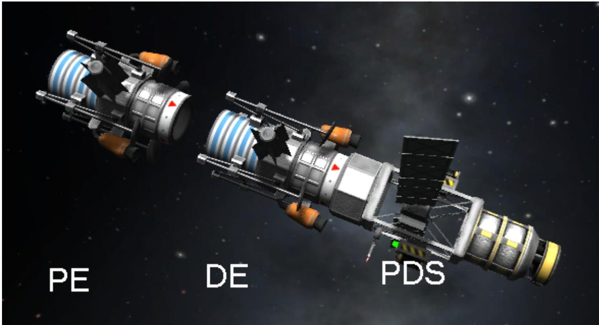
Figure 2: Artist's impression of the precursor mission: Deimos Explorer (DE), Phobos Explorer (PE), Phobos-Deimos Surveyor (PDS) satellite. PDS is equipped with solar-electric propulsion.
