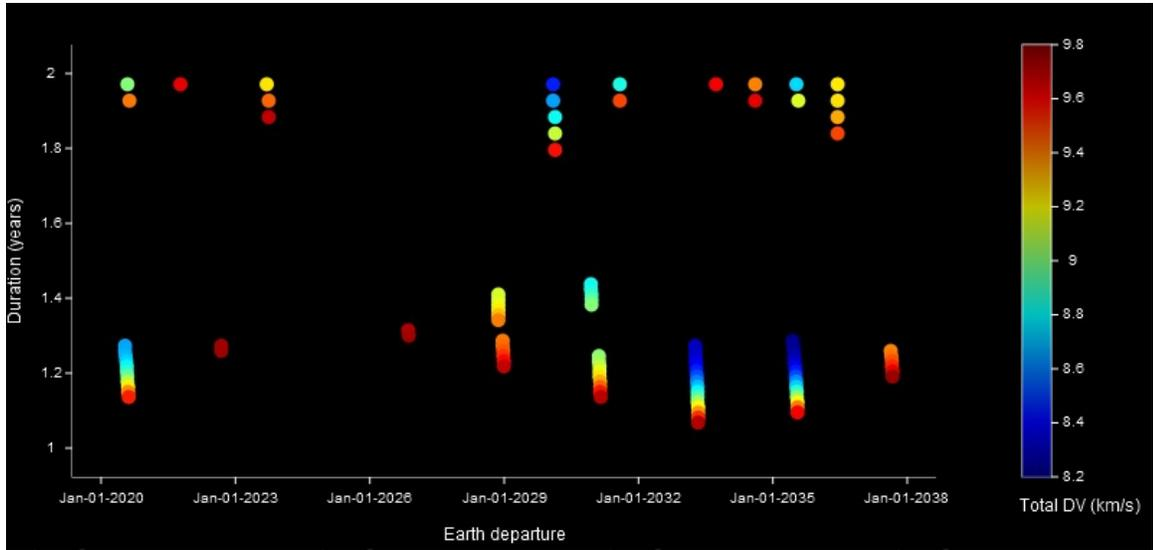
Figure 15: Total delta-v from LEO as a function of the Earth departure date and round-trip duration (Ames, 2013).
