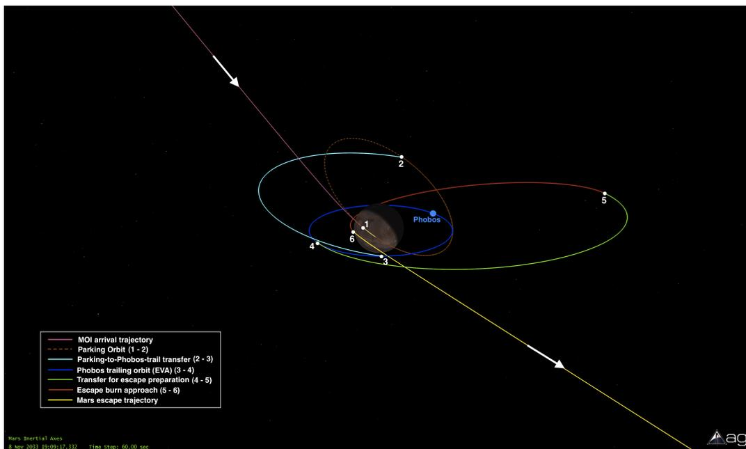
Figure 12: Alternative view of Areocentric trajectories, showing plane-changes for MOI and Phobos trailing orbit.
