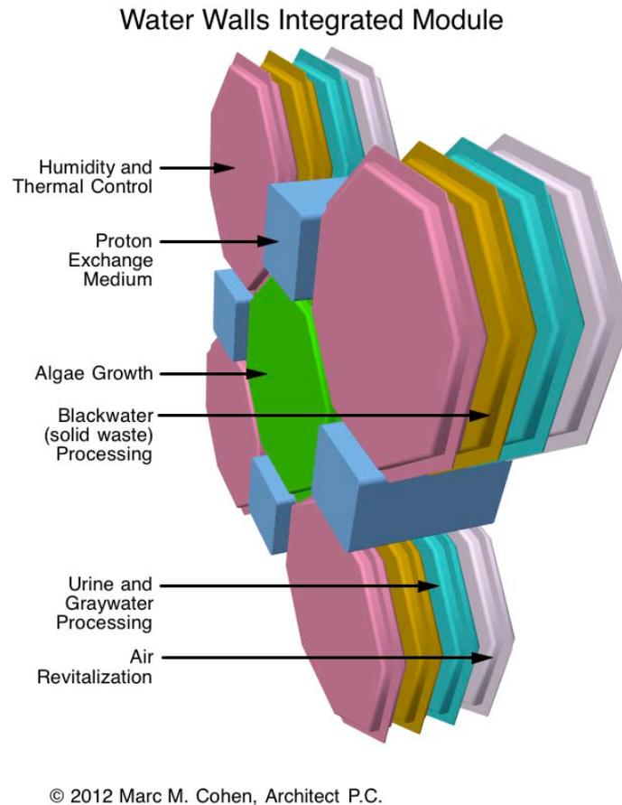
Figure 27: Water Walls FO Bag System Structure [Cohen and Flynn, GLEX 2012]
