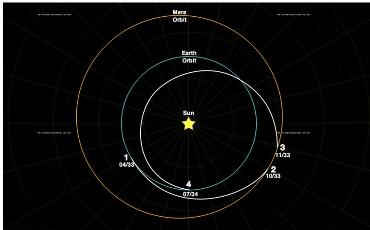
Figure 9: View along the ecliptic plane normal displaying heliocentric trajectories. The Earth-Mars trajectory connects points 1 and 2. The Mars-Earth trajectory connects points 3 and 4.
