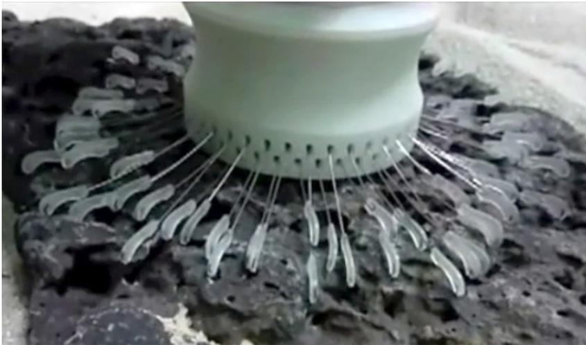
2. Adhesive feet, such as those in development by Northrop Grumman for the Automated Walking Inspection and Maintenance Robot (AWIMR) project.
