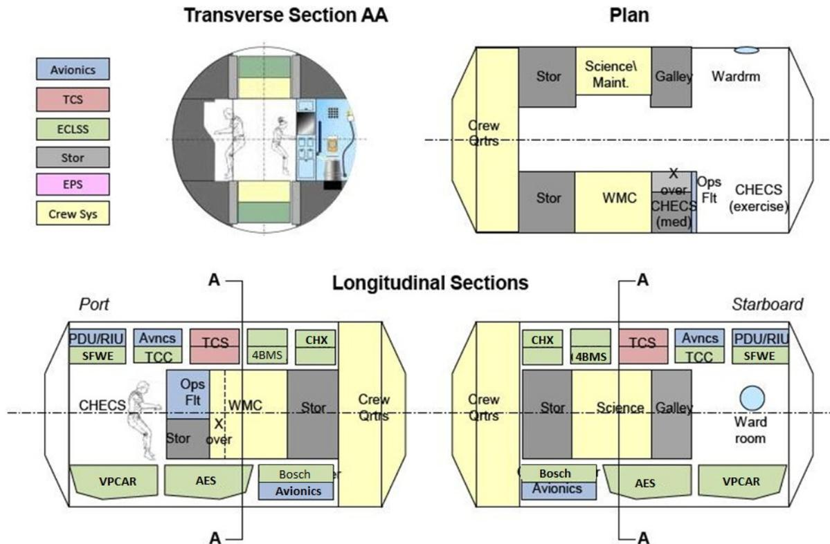
Figure 22: DSH Internal Layout of MPLM, Airlock and Node (Smitherman 2012)
