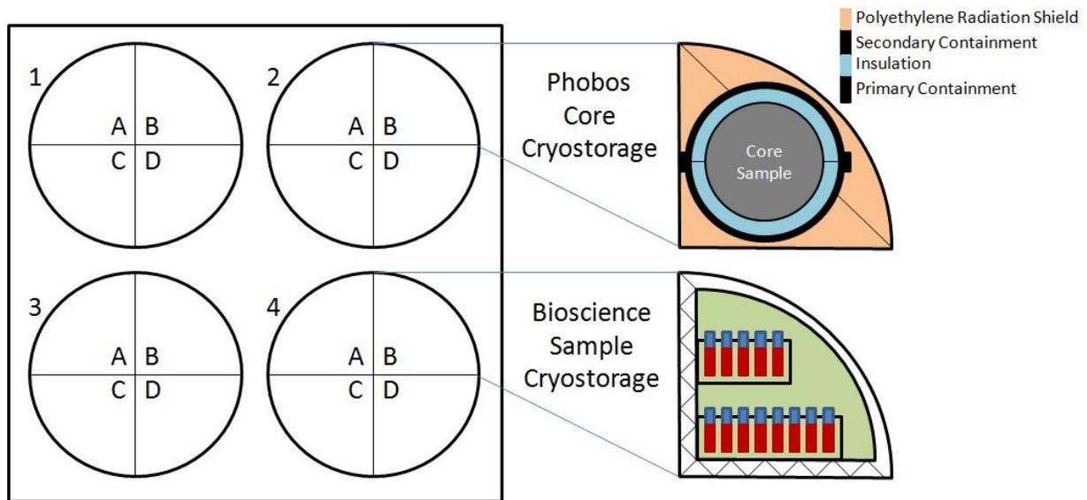
Figure 38: Schematic diagram of the sample storage locker configuration on the SEV. A similar locker configuration will be on the DSH for the return transit to Earth.
