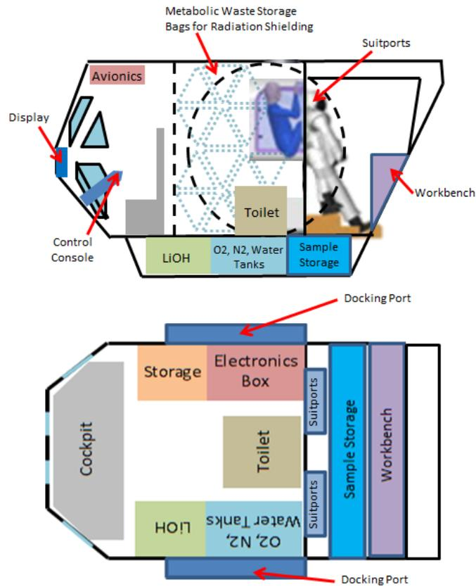
Figure 30: SEV Notional Plan View, Side View (above), Top View (below). Note the configuration by which a crewmember enters a spacesuit via a suitport in the top figure
