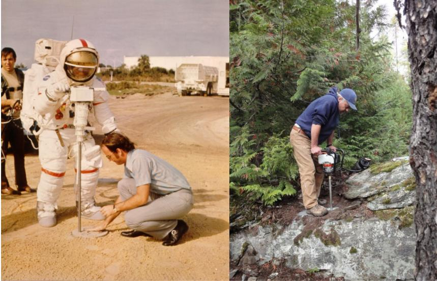
Figure 37: Examples of prototype portable drills to be used in space. (left) Example of the drill used on Apollo 15, 16, and 17 missions (<http://www.hq.nasa.gov/alsj/a15/a15carrier1.jpg>); (right) Commercial “backpacker drill” sold by Shaw Tool Company used for mineral prospecting in remote locations. This gasoline-powered drill would need to be retrofitted with an electric motor. (<http://www.backpackdrill.com/images/home003.JPG>; image care of Shaw Tool Co.)
