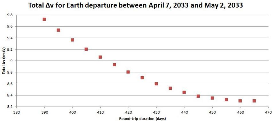
Figure 16: Total  $\Delta v$  requirements for Earth departure between April 7, 2033 and May 2, 2033.
