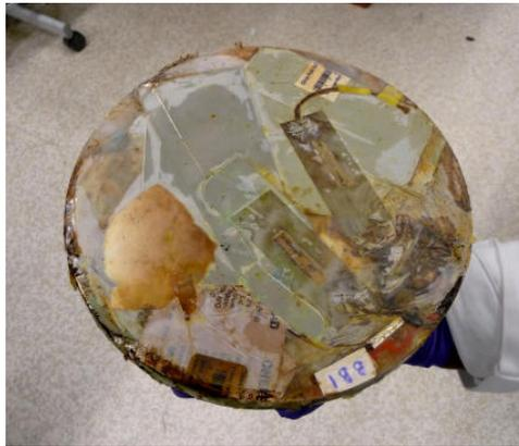
Figure 24: Example of a waste “puck” produced by an experimental Heat Melt Compactor
