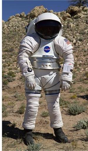
Figure 31: NASA Mark III EMU (with PLSS designed to interface with suitport)
