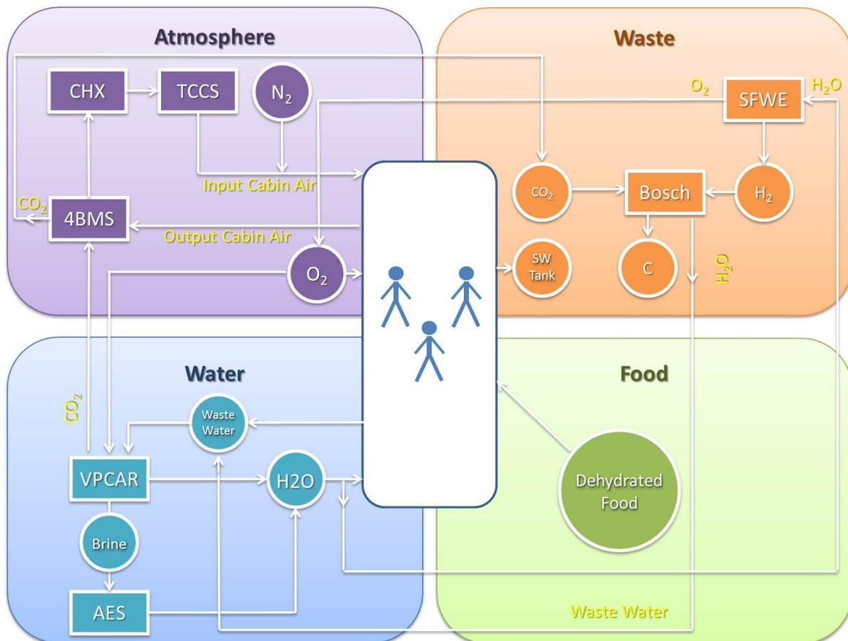
Figure 23: DSH Primary ECLSS Flow Diagram
