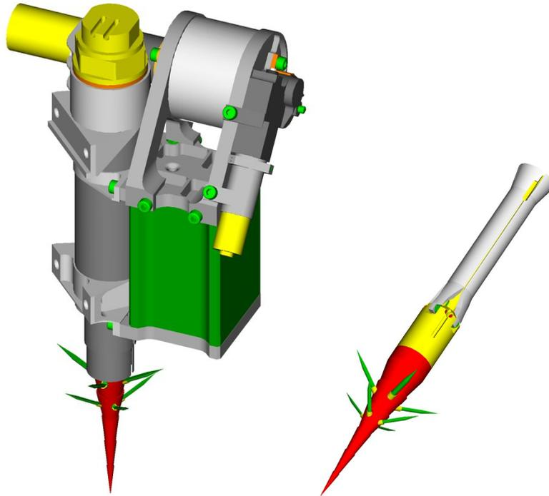
Figure 33: CAD drawing of representative anchoring harpoon for a lander, from Rosetta's Philae lander.
