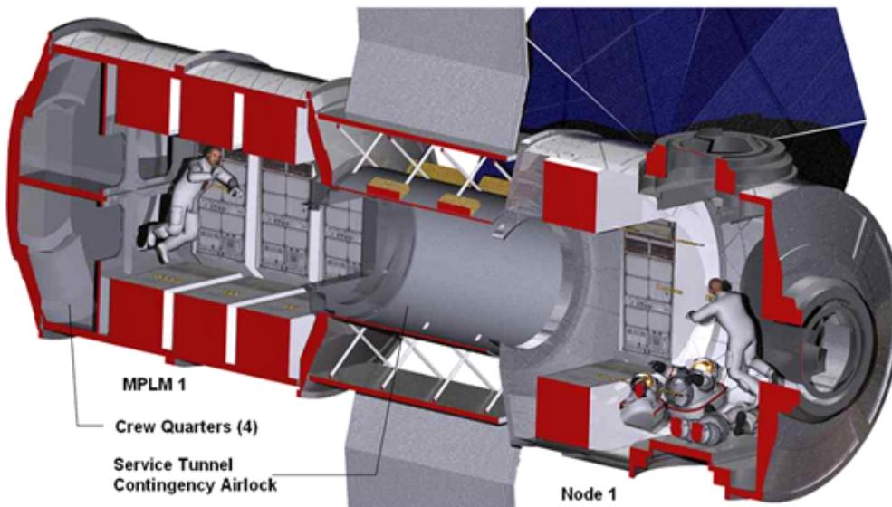
Figure 21: Deep Space Habitat MPLM and Node Internal Structure (Smitherman, 2012)
