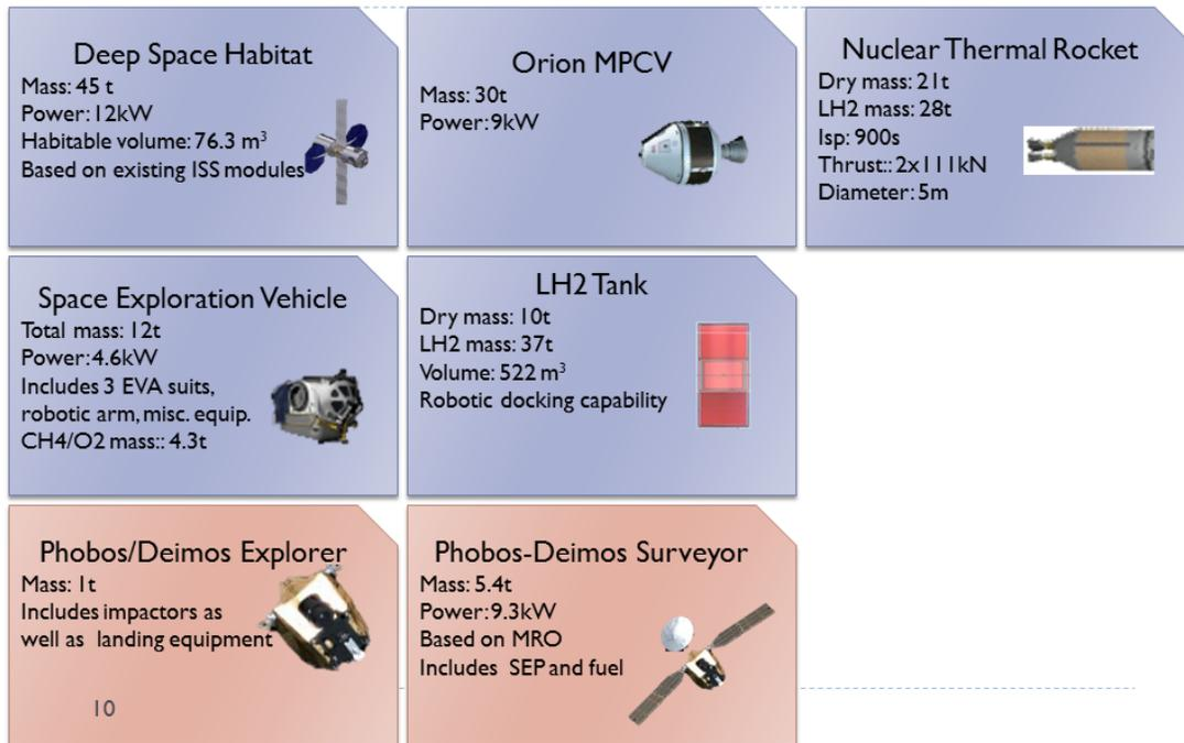
Figure 8: Building blocks of the Asaph precursor and main mission
