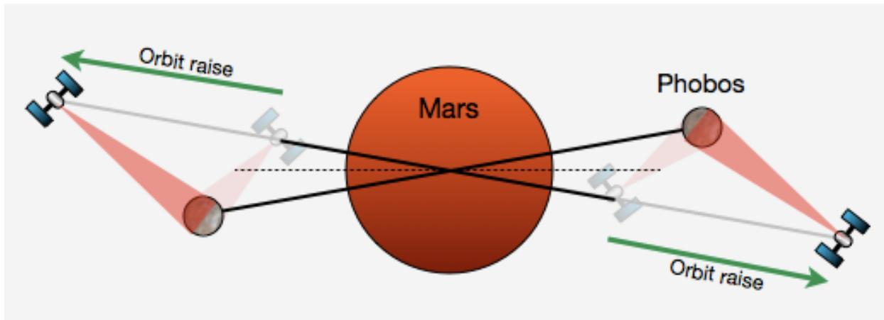
Figure 6: The two orbits used to image over 80% of the surface of Phobos are displayed. The first orbit (grayed) has an altitude of 9000 km, while the second has an altitude of 9700 km.
