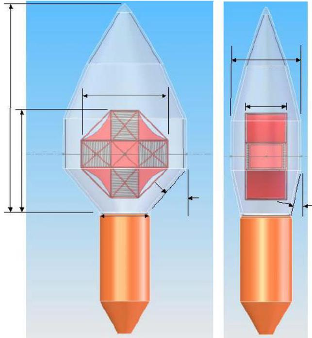
Figure 18: Initial payload fairing design
