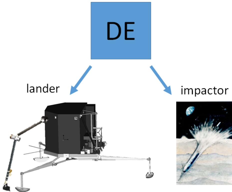
Figure 5: The Deimos Explorer (DE) separates into an impactor (activates first) and an immobile lander (activates second).
