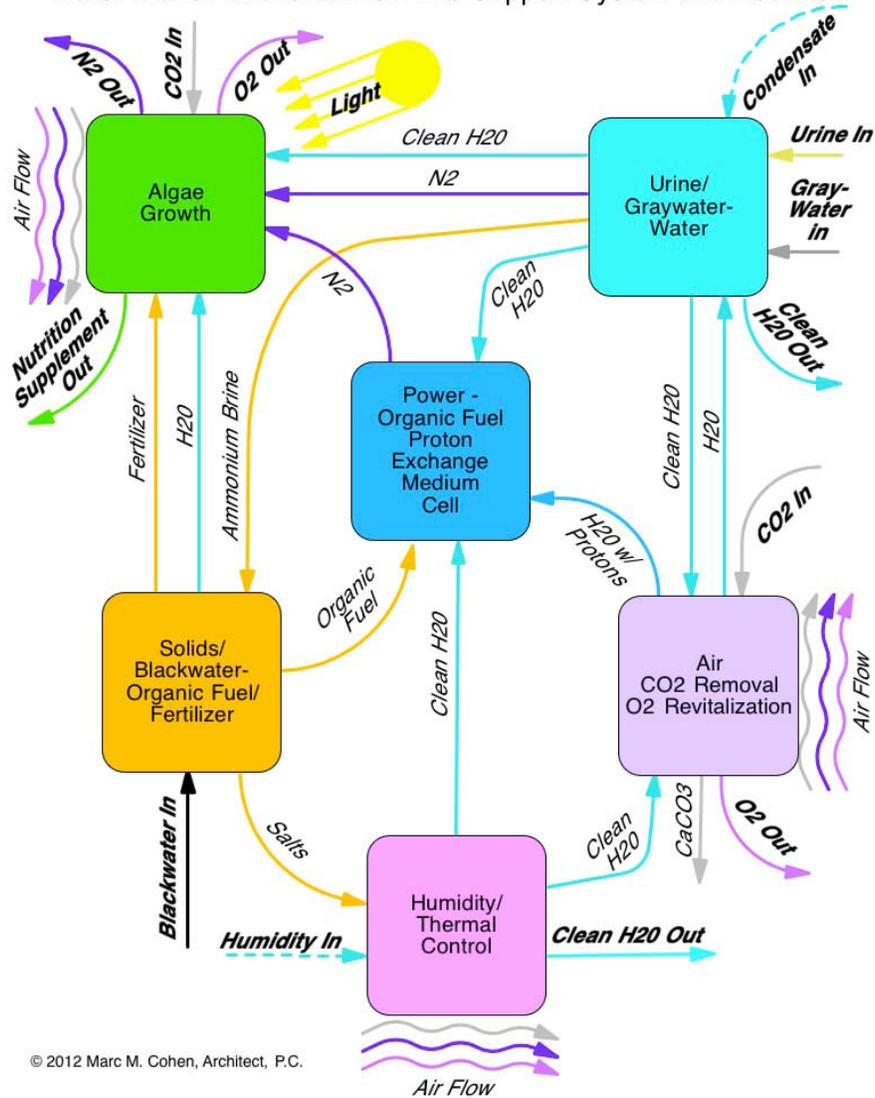
Figure 28: Water Walls Mass Flow Diagram [Cohen and Flynn, GLEX 2012]
