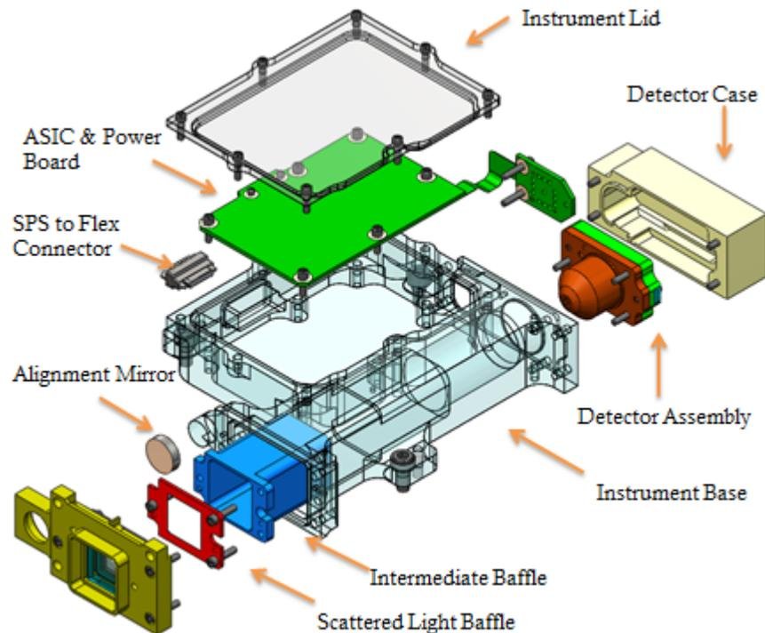
Figure 40: Exploded view of GOES-SPS
