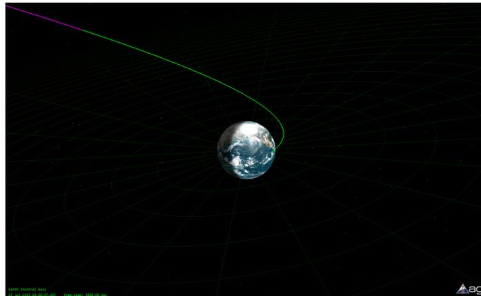
Figure 10: Earth escape trajectory with an outgoing asymptote right ascension of  $272^\circ$ , declination of  $-23^\circ$ , and velocity azimuth at periapsis of  $90^\circ$  in the Earth inertial reference frame.
